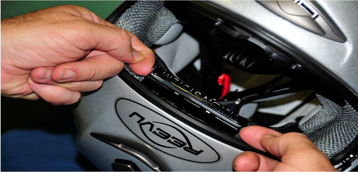
Fig 2. Clip nail under Vision system cover and pull free
